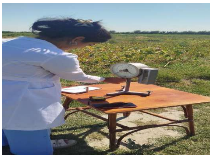
Rasm. Soya navlarini transpiratsiya jadalligini BT-500 torsion tarozida o'rganish jarayoni
