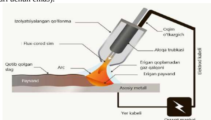
4-rasm. Flux-Cored Arc payvandlash (FCAW) jarayoni
