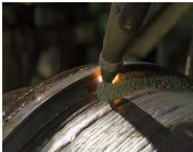
4-rasm. Kukun ostida payvandlash jarayoni
