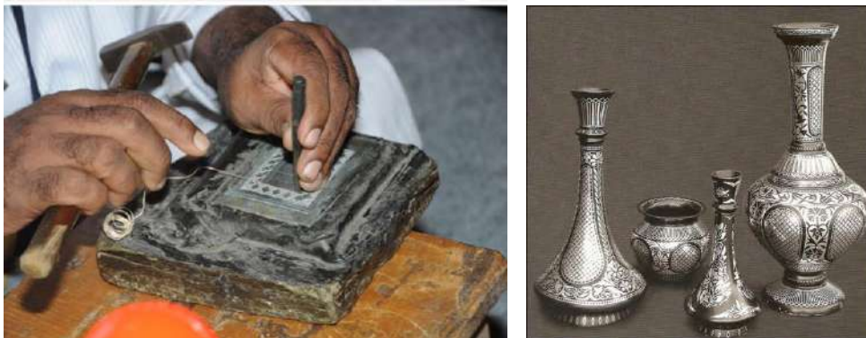
4-rasm. Hindiston “Bidriware” (Bidar shahriga xos) mis buyumlarni o’yish jarayoni
