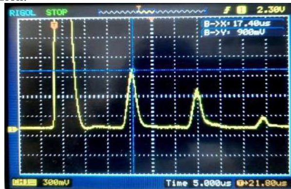
Fig.2. An image of a series of echo pulses with a delay interval relative to each other
